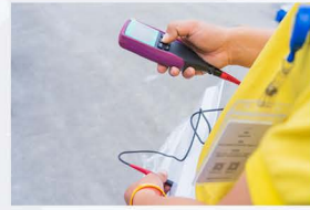
STEP 2 FILM THICKNESS GAUGE
